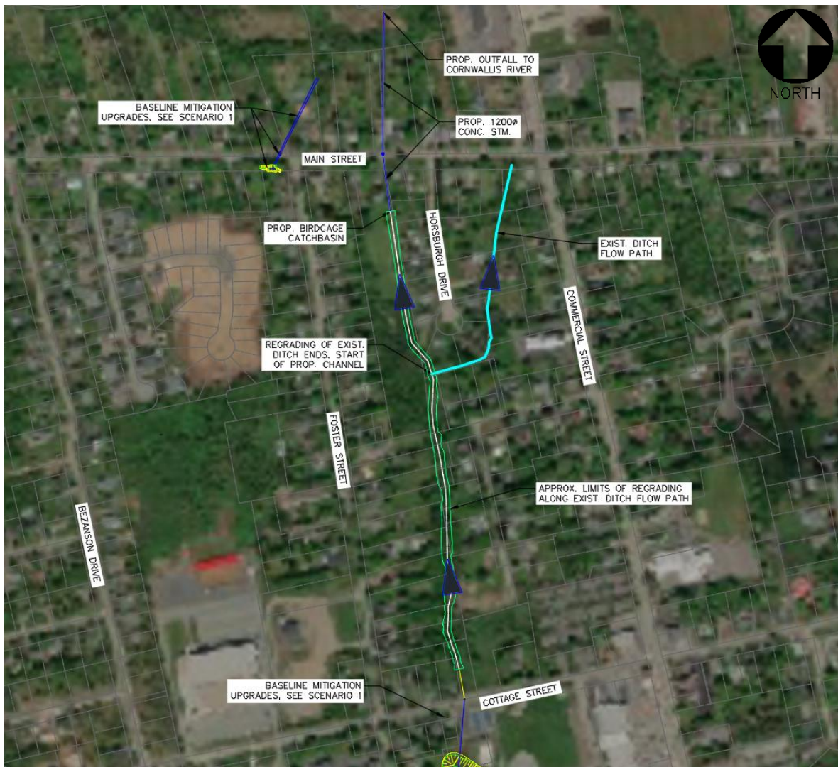
Figure 4-11: Sketch of the Channel Diversion
