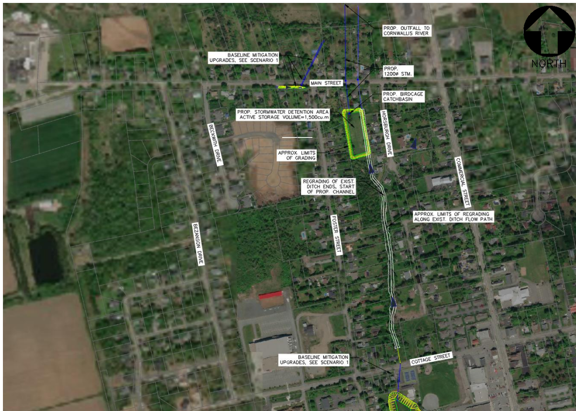
Figure 4-13: Proposed Grading Extents of Secondary Detention Area
