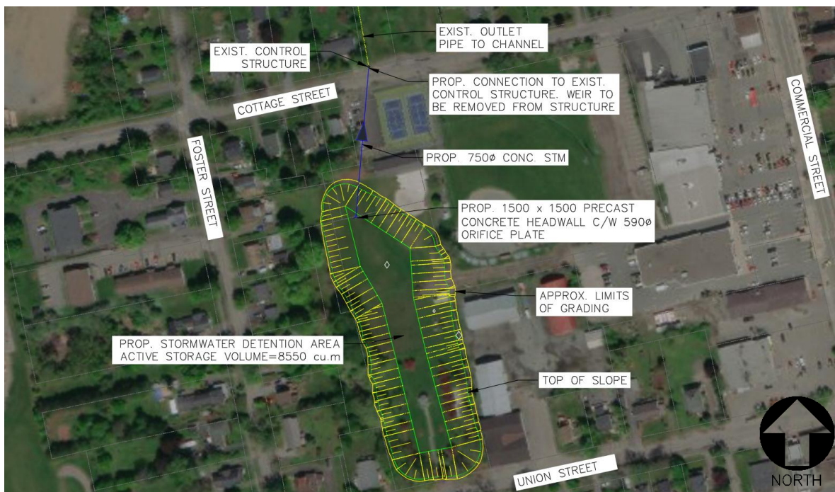
Figure 4-2: Centennial Park Detention Area Details
